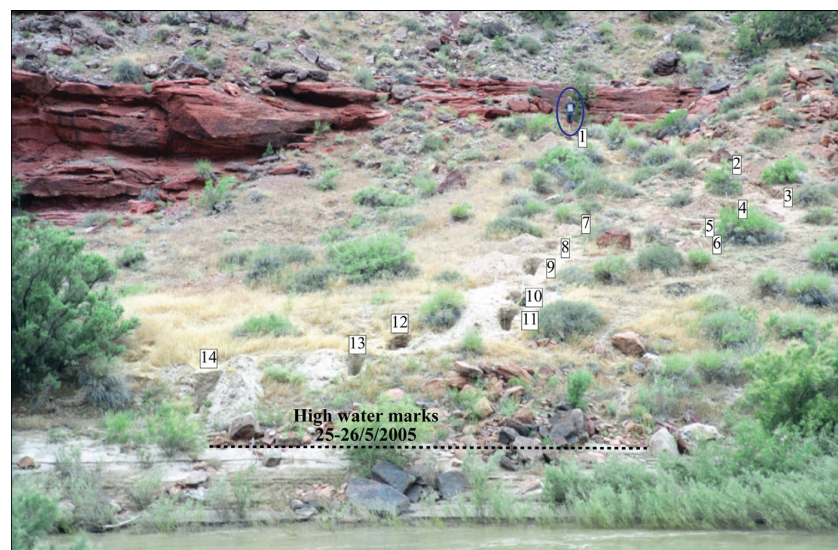
Figure 7. Paleoflood slackwater deposits at the study site. The numbers represent the stratigraphy pits. Pit no. 1 (with a nearby person for scale) is the highest flood deposit—about 15 m above the water surface ( 425 \text{ m}^3 \text{ s}^{-1} , June 2005). Note the high water marks of the observed 25–26 May 2005 flood—peak discharge of 1140 \text{ m}^3 \text{ s}^{-1} [Greenbaum et al., 2006b].
