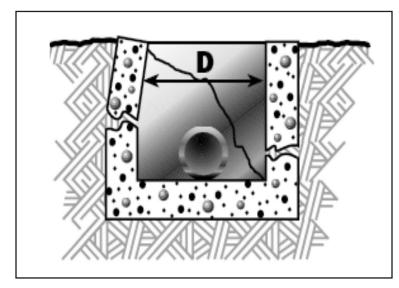
Figure 33—Failure of a concrete outfall structure.
