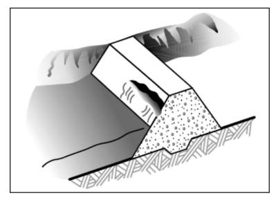
Figure 7—Slide, slump, or slip.
