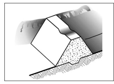
Figure 23—Low area in the crest of a dam.
