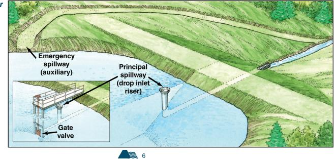
Figure 4—Typical drop inlet riser serving as a principal spillway to control water level.
