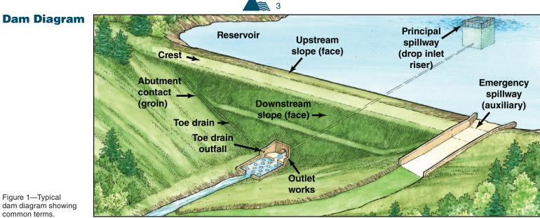
Figure 1—Typical dam diagram showing common terms.
