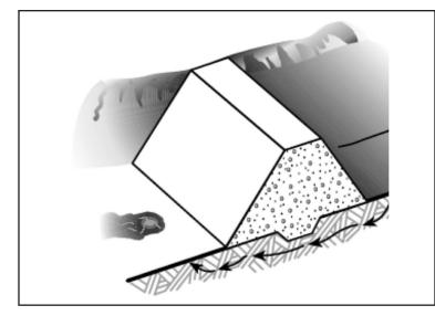
Figure 27—Seepage water exiting as a boil in the foundation.
