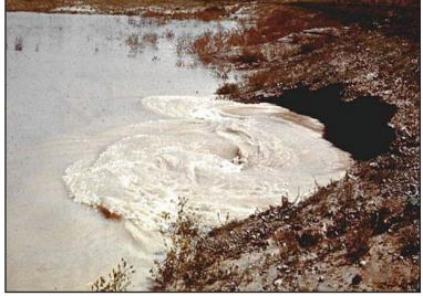
Figure 6—Whirlpool action is an indication of advanced piping.
