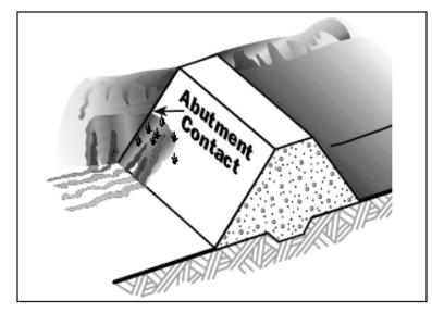
Figure 29—Seepage exiting at the abutment contact (groin).
