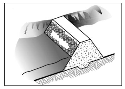
Figure 9—Broken down or missing riprap.
