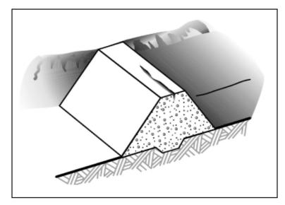
Figure 21—Longitudinal crack.
