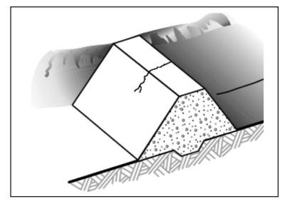
Figure 19—Transverse cracking.
